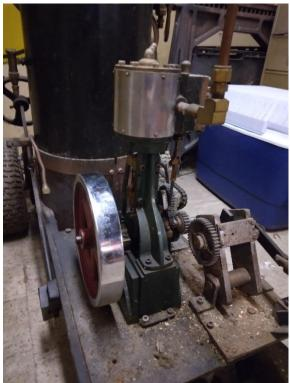
This is a free lance tractor driven by what looks like a Stuart vertical engine. Boiler is a dry bottom fire box. Chain drive. There is a small water tank trailer that goes with it.
